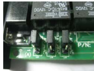
Figure 4: Jumper position for closer (AC)
