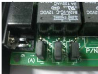
Figure 3: Jumper position for opener (AO)
